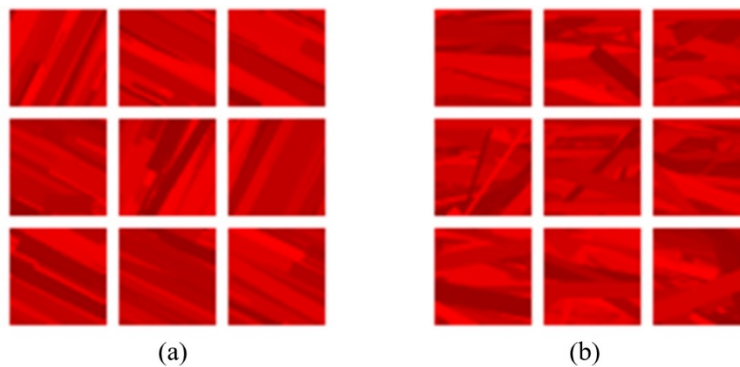
Fig. 8. Example of model data: (a) – organized fibers, positive samples, (b) – disorganized fibers, negative samples.
